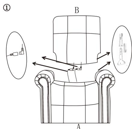
1. Connect the connector of back and seat
