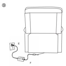
3. Connect the connector from motor to the power cord and transformer
